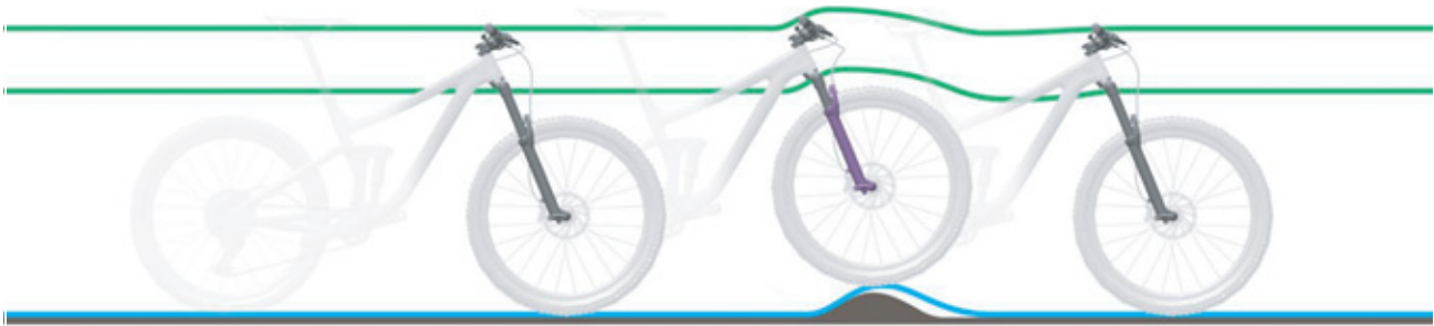
Figure 211: Excessively hard damping in the suspension fork on bumps
