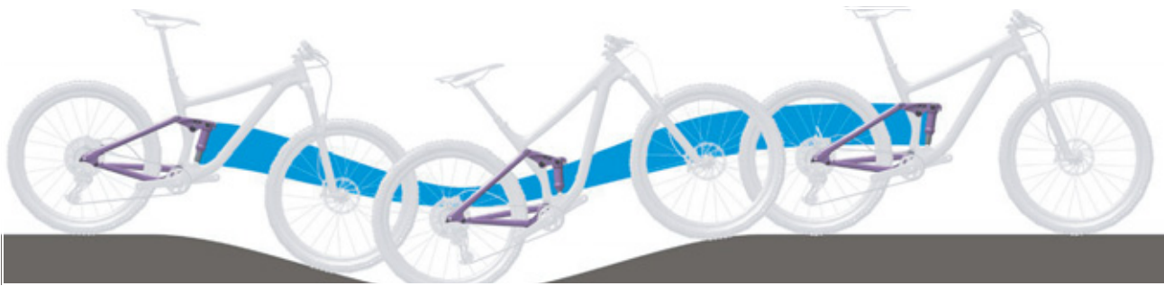
Figure 225: Excessively soft suspension in the rear frame damper on hilly terrain
