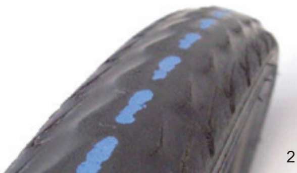
Figure 162: Tyre without tread which can be replaced (1) and tyre with puncture protection showing through (2), which must be replaced
