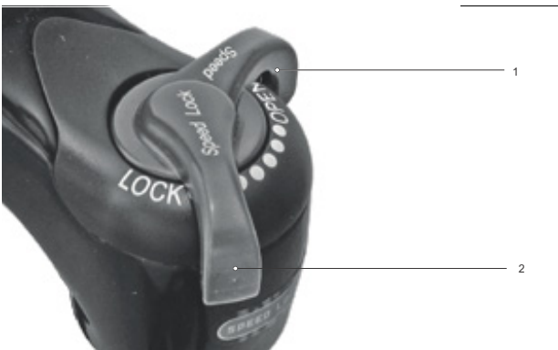
Figure 202: Changing compression adjuster to a harder setting
