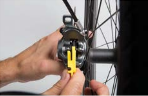
Figure 164: Checking the brake lining when fitted with the help of the transport safety wear gauge
