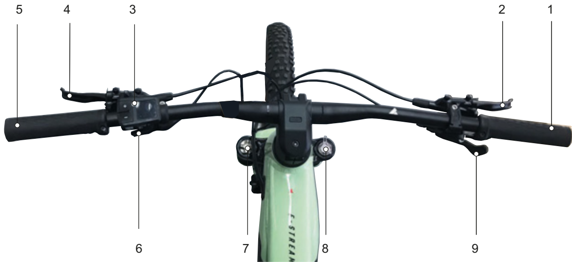
Figure 36: Detailed view of handlebars with FIT Remote LCD on-board computer, example
