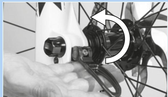
Figure 72: Pressing the quick release lever in the direction of the arrow
