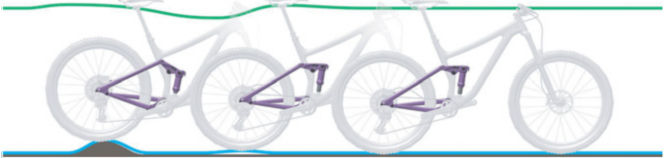
Figure 213: Rear frame damper rebounding too quickly
