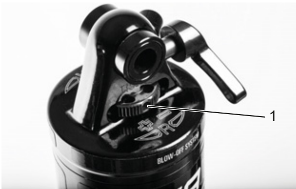
Figure 214: SR SUNTOUR rebound adjuster wheel (1) on the rear frame damper
