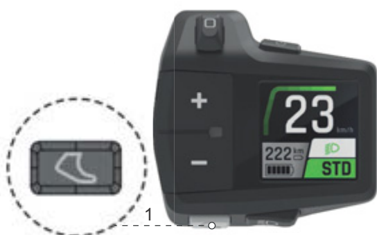
Figure 146: Position of push assist button
