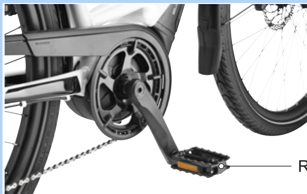
Figure 86: R-pedal in the right-hand crank arm
