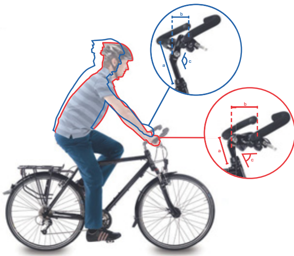
Figure 114: City bike (blue) and trekking bike position (red) by changing the angle
