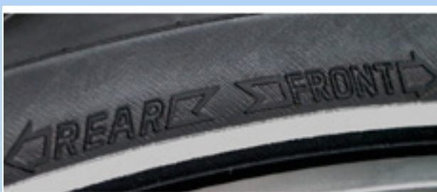
Figure 64: Rotation direction arrow on MTB tyres
