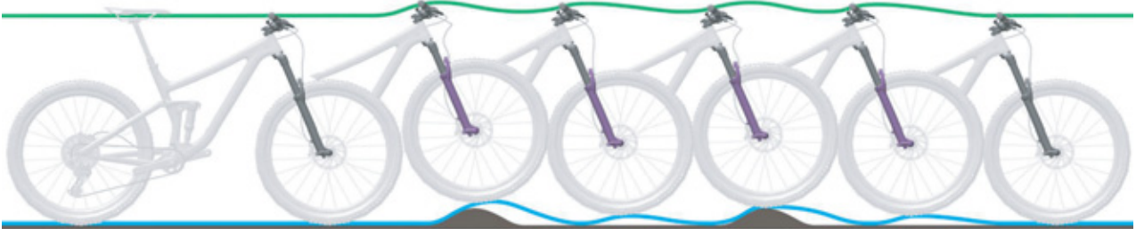
Figure 205: Suspension fork rebounding too quickly
