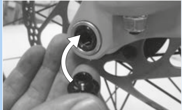
Figure 67: Inserting the securing screw
