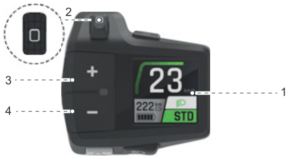
Figure 38: Display (1) on the FIT Remote with LCD
