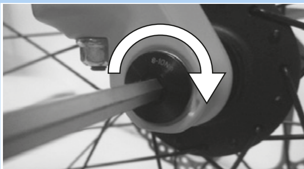
Figure 66: Tighten the axle in the direction of the arrow
