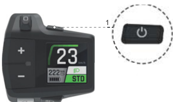
Figure 130: Display (1) on the FIT Remote with LCD
