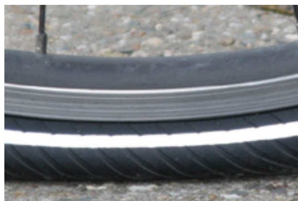
Figure 117: Much too little tyre pressure
