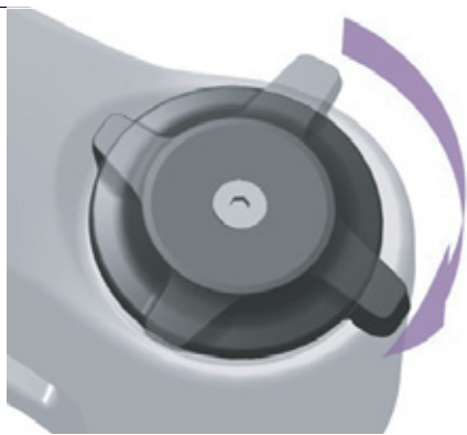
Figure 210: Changing compression adjuster to a harder setting
