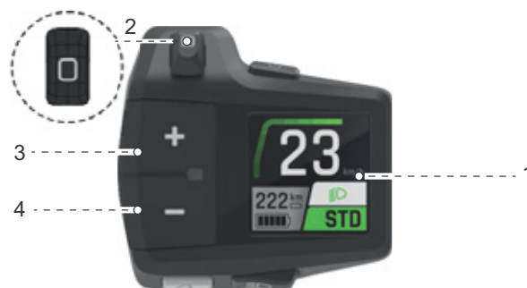
Figure 131: Display (1) on the FIT Remote with LCD
