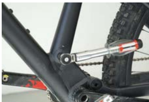
Figure 100: Tightening the seat post axle
