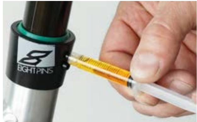
Figure 160: Lubricating the eightpins seat post
