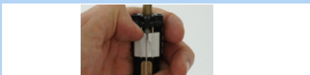
Figure 156: Pushing the white activation slider downwards
