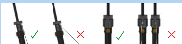
Figure 157: Correct and incorrect Bowden cable
