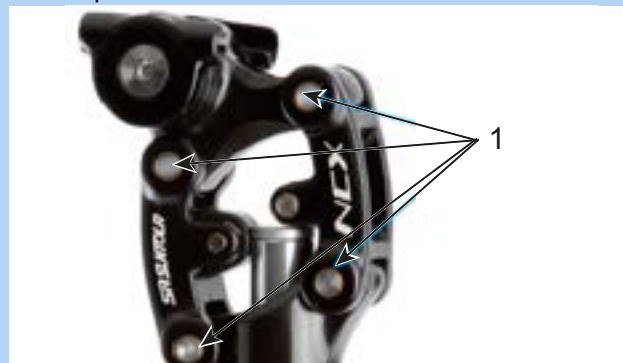
Figure 129: SR Suntour suspension seat post lubrication points
