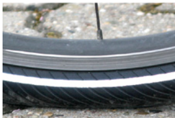
Figure 74: Correct tyre pressure. The tyre is barely deformed under the load of the body weight
