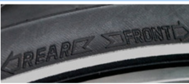
Figure 51: Rotation direction arrow on MTB tyres
