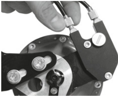
Figure 123: The tension adjuster on Rohloff hub versions with external switch control is located on the cable box positioned on the left-hand side
